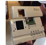
PPJ Engineering Split type A/C system with energy saving system already installed. (25 Plus series Econo-Thermostat). This energy saving system aims to regulate in a more efficient way the refrigerant pressures and save about 15% energy.
