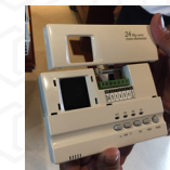
PPJ Engineering Split type A/C system with energy saving system already installed. (25 Plus series Econo-Thermostat). This energy saving system aims to regulate in a more efficient way the refrigerant pressures and save about 15% energy.
